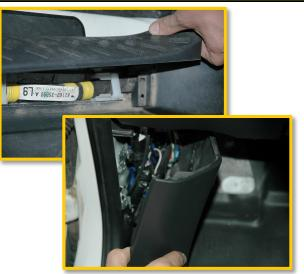
13. Unscrew and remove gear shift selector knob and e-brake cover.
