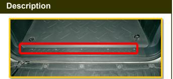
2. Remove two front cargo hooks and remove trim.
