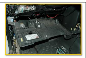
16. Remove drivers AC vent cover by pulling up and out.
