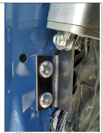
Your DRILL Marks should be Right in line where the Vapor barrier Black Tacky strip was on the door.
