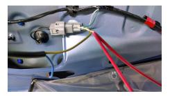
Note On Actuator wiring. Some version of the Actuator came with Brown and Blue lead wires, others came with Red and Black. Use this as your connection rule. The Brown or Red wires are your positive wire to move the actuator UP. These colors need to be connected to the RED leads of the Wire Harness AND the GREEN wire on the Window Pop
