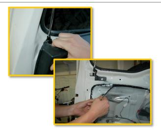
7. Open the rear left cubby if you haven't already. Unclip the rear door wiring harness by pulling the clips from the body. Disconnect the harness. Disconnect washer fluid hose also located in the rear left cubby.
