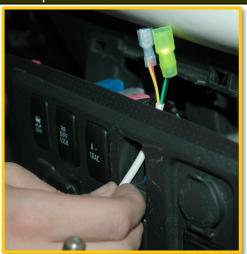
Run harness behind the center console stack and knee panel area. Secure the harness as necessary. Run harness under the driver's rocker panel. Use the factory clips to retain the harness. Run the harness behind the driver's rear panel.
