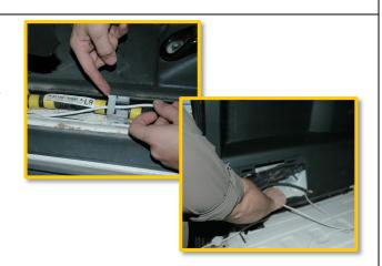
4. Cut rubber sheathing around wiring body grommet. Run harness out the vehicle body wiring access hole and through the boot. Take your time to run the harness as to not damage the wire. Run harness through rear door wiring access hole. Pull the harness all the way through the boot and then reinstall the boot grommet to the rear door and body. Reconnect the door wiring harness and washer tube.
