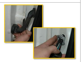
Disconnect window latch wiring harness and unclip from the rear inner door panel. Using a razor blade, slit wiring harness sleeve. (BLACK)
