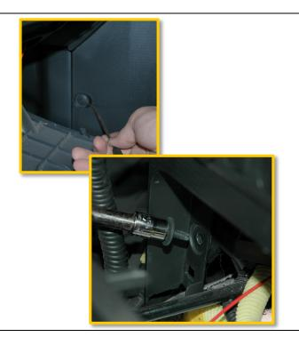
18. Pull out plate and remove a blank switch cover.
