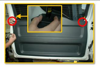
Unlatch rear window by using your key and fully raise rear window. Pull on rear hatch cover and unsnap the entire cover and remove. Pull back the vapor barrier. Take care with the barrier adhesive.
