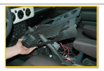
14. Remove four 10mm bolts from center console. Slide center console as far back as it will go.
