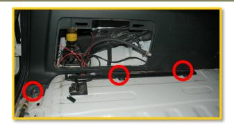
Remove two screw covers and screws from rear hatch door cover.
